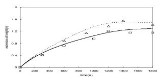
Figure 5. Height extension during baking with convective heating ( $\Box$ : experiment; solid line: model) and combined microwave–convective heating ( $\Delta$ : experiment; dashed line: model).
