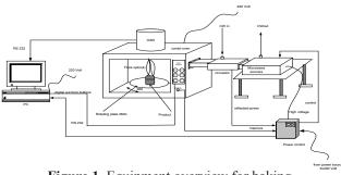
Figure 1. Equipment overview for baking
