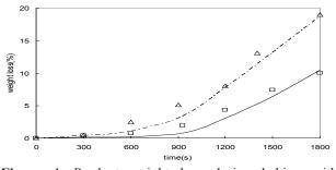
**Figure 4.** Product weight loss during baking with convective heating ( $\Box$  : experiment; solid line: model) and combined microwave–convective heating ( $\Delta$ : experiment; dashed line: model).
