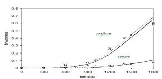
**Figure 8.** Color developments during baking in the center of the product and at the crust. Results for convective heating ( $\Box$ : experiment; solid line: model) and combined microwave–convective heating (O: experiment; dashed line: model).
